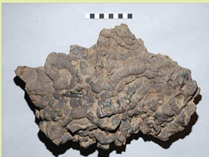
*A large slab of early iron slag showing the characteristic flow patterns; the scale is 10cm. Photo: author.*
